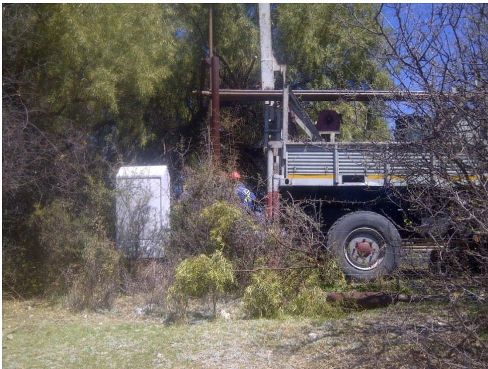
Figure 40: Aquifer Testing of Existing Borehole SD1-GAA001
